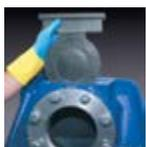
A positive sealing, externally removable suction check valve is standard on Ultra V Series® models. This eliminates the need to disconnect any piping for inspection or replacement. The check valve has a blowout center that limits excessive volute pressure, protecting the pump.
