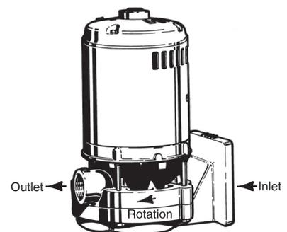
to Section 1, 1C Placing Stored Pumps Into Service. Because of the large areas of close fitting surfaces inside these pumps, it takes only microscopic residue to produce substantial resistance to rotation. Once loosened, this material is quickly dispersed and the impellers find their hydraulic center. If these procedures are followed carefully, no damage will result from "breaking loose" the impeller.
