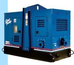
The modular design, featured on several PA Series® pump models, enables the addition/removal of a lightweight, aluminum, acoustically-treated enclosure to the standard fuel base. The enclosure provides excellent corrosion resistance and offers a significant reduction in sound levels (68 dBA at 23').
